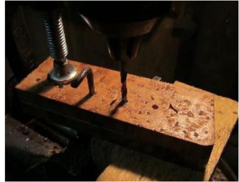
You can now use the holes on the second scale and two or more pins to locate the tang for tracing of outline on to that scale. Like the first one, white pencil followed by black works well (especially on dark, highly figured woods).
