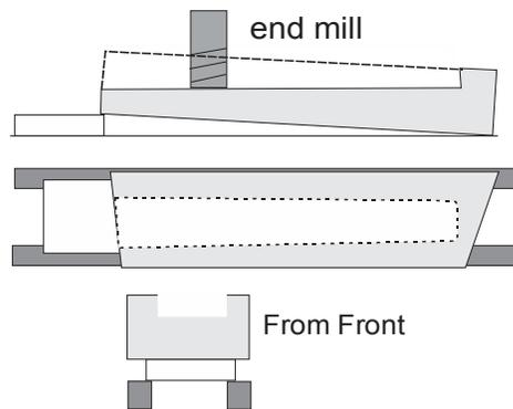
If there is an appreciable taper across the tang at the front (top of tang to bottom of tang), shim the top of the handle appropriately
