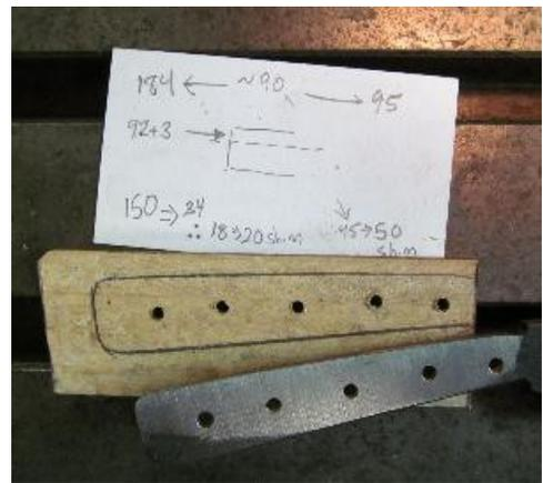
Finally clamp the two scales together around the tang and verify that there are no gaps. If there are, you will have to deepen the recesses until the gaps vanish.
