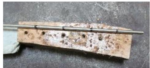
The pin stock is sheared (here using a re-purposed fencing tool). The shear will crush the ends of the pins which is why a bit of extra length is needed. One end will be given a slight point on the knife grinder.
