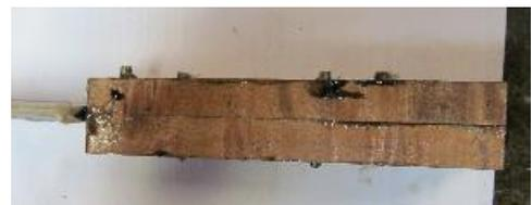
The rationale for the excess pin length is shown with a quick grind. The pins show a round and complete profile. Note that #3 does not have a pin yet.
