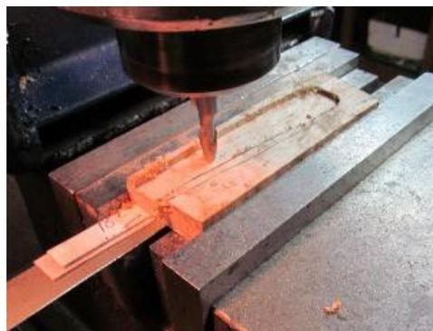
The final adjustment is done with a 1/8" air die grinder and a small cutting bit. The tang is laid on the recess and the location where a bit more wood needs to be removed is determined. Do that and repeat until the tang snaps into the recess. Be sure to match the curve at the bottom of the shoulders.
