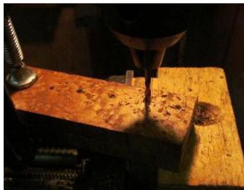
C-clamps and drill chucks often compete for the same physical location, so move the clamps and pins as needed.
