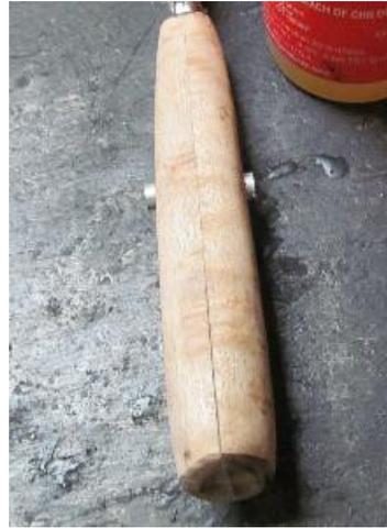
After buttering the pins, use the vise to drive pins home. Be careful to run them in without splitting the handle!
