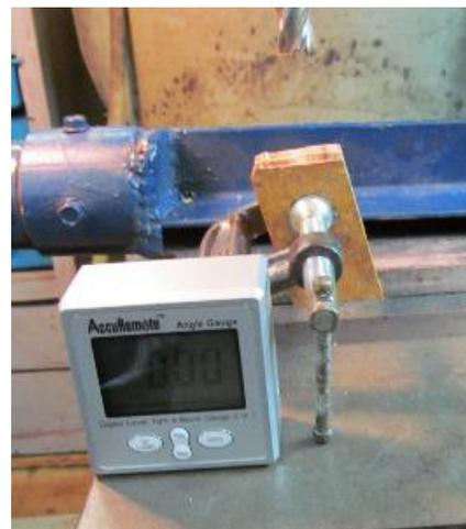
The protractor is placed on the end to be flattened. The blocks are gently tapped in the appropriate direction until the protractor indicates zero. The vise is closed fully and...
