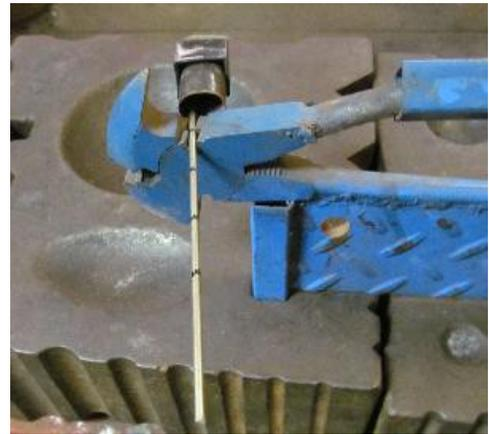
The pins are gently started in the holes. Note the tapered pin end. That end goes in first and will help align the pin without splintering the far side of the second scale.
