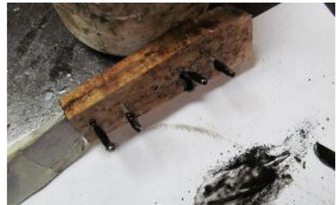
Use a mechanic vise to drive pins. The rear jaw has a liner made of 3/4" plywood. As the pins emerge from the back of the 2<sup>nd</sup> scale, the liner will support the scale while the pins penetrate the plywood.
