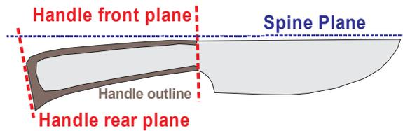
Since the goal is to create a cavity inside of the handle that very closely matches the tang, the process must accommodate any taper from front of tang to rear and any differences of thickness from top of tang to bottom. Sooo...
