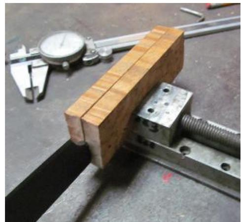
It is now glue time. You will need gloves, masking tape, 5-minute epoxy, epoxy colorant, 2 alignment pins and three C-clamps. The colorant I use came from Brownell's but is no longer available. A quick web search turned up "Castin' Craft Opaque Pigment 1 Oz: Black" which might do or even laser toner could suffice (if you can control that stuff!).
