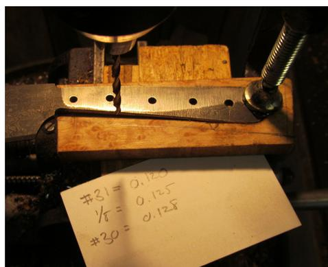
One of the realities of smithing (and knife making) is figuring out how to hold things. While C-clamps work, they are bulky. Old lab hose clamps actually work quite well. Alignment pins are very useful and are made from pin stock bent into 'L's and slightly ground to fit the #31 holes.
