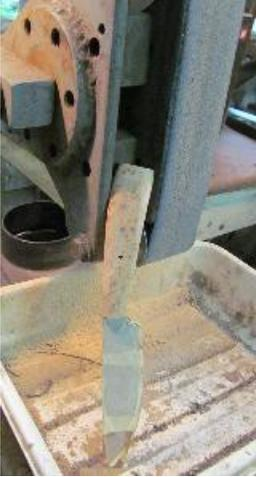
A close-to-finished profile is generated using a slack belt setting of the grinder.
